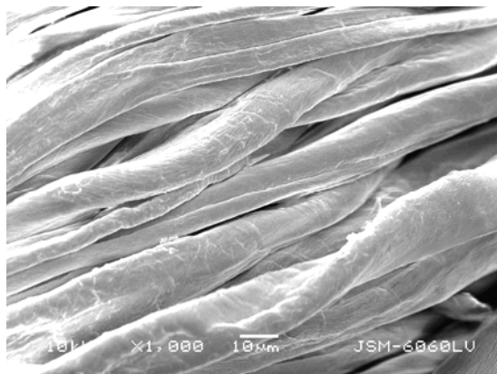
Figure 1. Cotton fibres impregnated with 3M ZnCl_2 .
